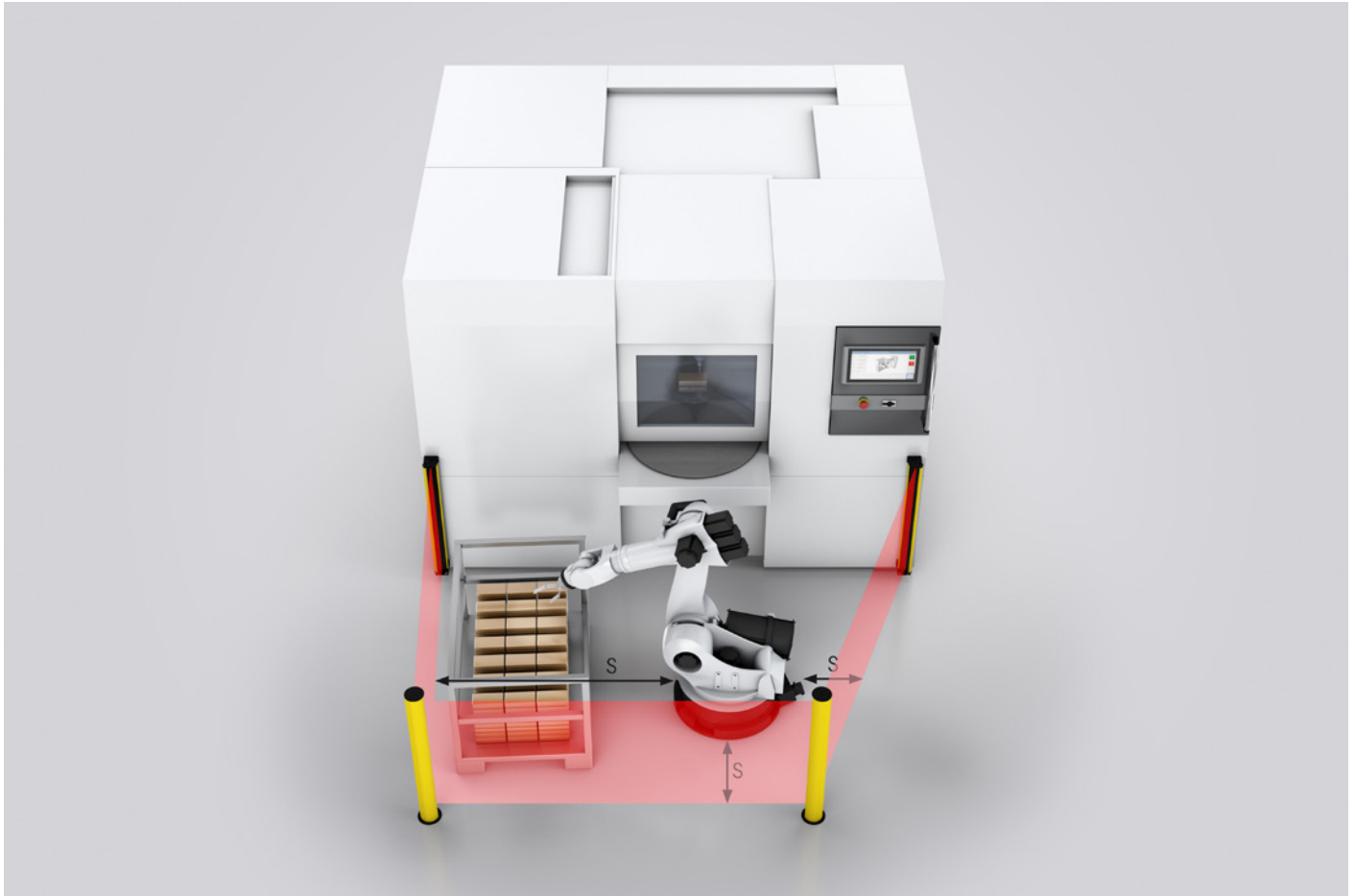
Figure 5: Safety distance S
