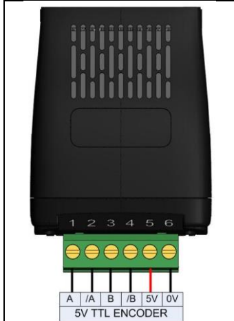
Connection Example – 5V TTL Encoder OPT-2-ENCOD-IN
