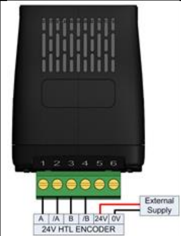
Connection Example – 24V HTL Encoder OPT-2-ENCHT-IN
